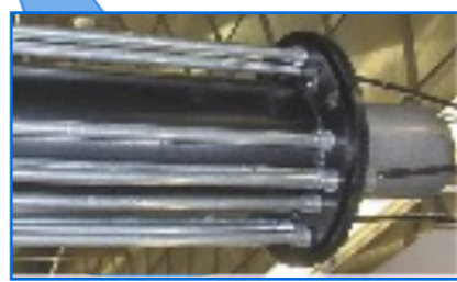
LUCID [Luminosity Monitor] Cherenkov gas tubes, at ~17 m from IP.
